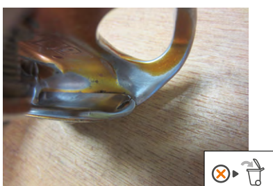
• Wear caused by rope running through the device.
